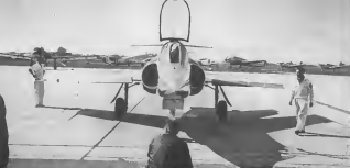
TAKING in with canopy lifted, the Douglas B-70 shows its small size, large feet for coping with rougher fields. Note leg and eye steps in two segments.
